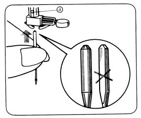
With flat face away from you, insert a new needle into groove of needle bar.
